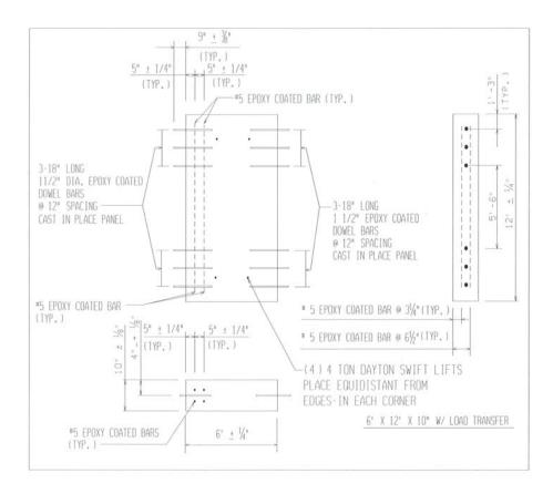
Figure 1. Structural details of the doweled precast panel.
