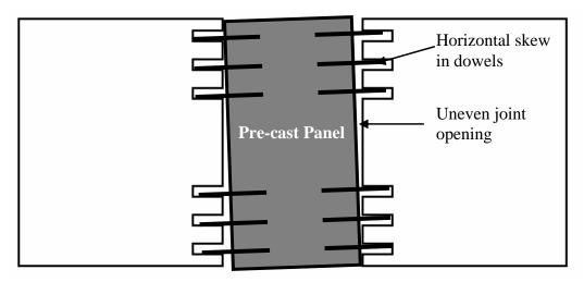
Figure 18. Line sketch illustrating the possible dowel skew and uneven joint opening.
