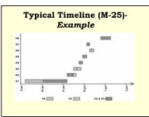
Example Gantt Chart illustrating time to complete the installation of two panels (multitasking and overlapping of activities).
