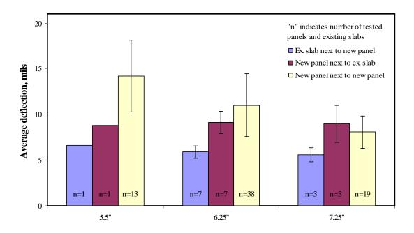
Figure 34. Average joint deflections (leave) as a function of slab thickness.
