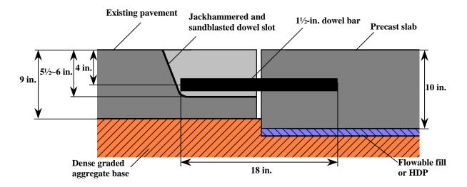
**Figure 7.** Schematic cross section of the dowel assembly.
