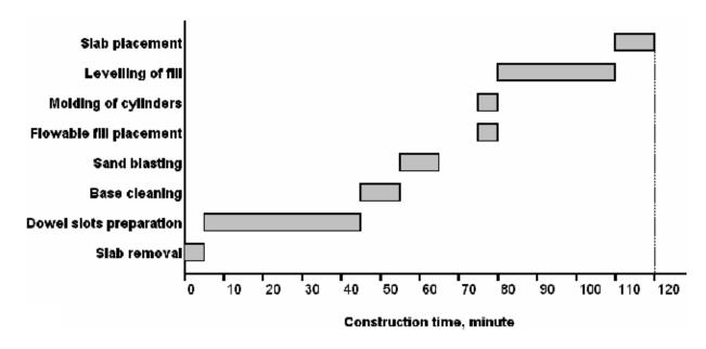
**Figure 11.** Construction timeline for panel 5.
