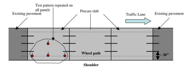
**Figure 30**. Falling-weight deflectometer testing pattern.
