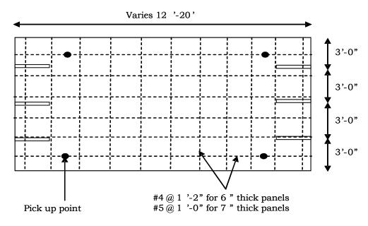
Figure 20. Structural details of the precast panel.
