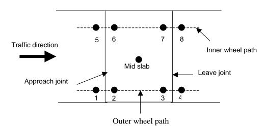
Figure 14. Falling-weight deflectometer test locations to evaluate panel effectiveness.
