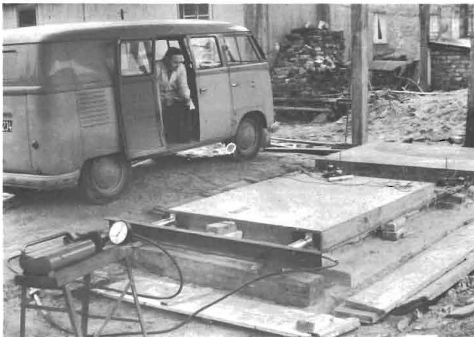
Figure 6: Test for determining the coefficients of friction between slab and base for various types of sliding layer.
